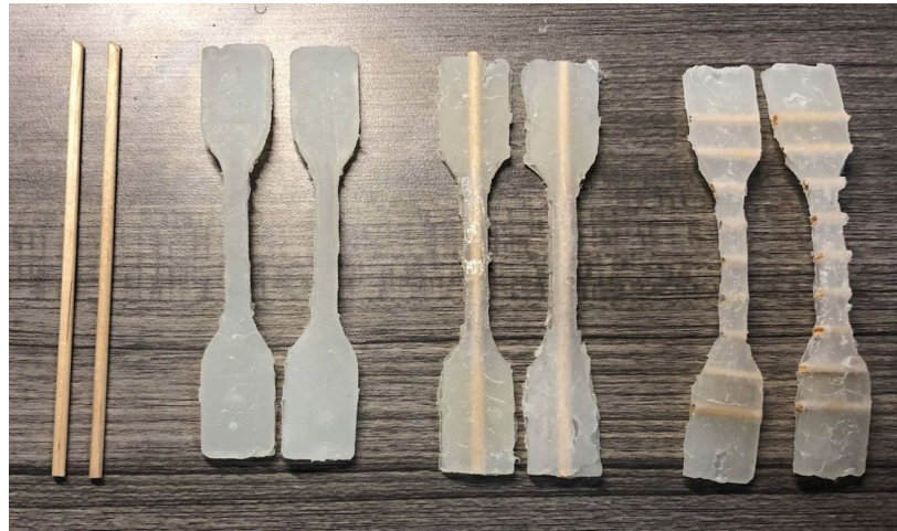
Figure 5: Items tested on Instron
