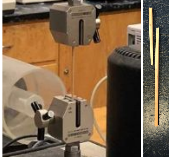
Figure 7: Fiber loaded for tensile test in process (left), failed fiber (right)
