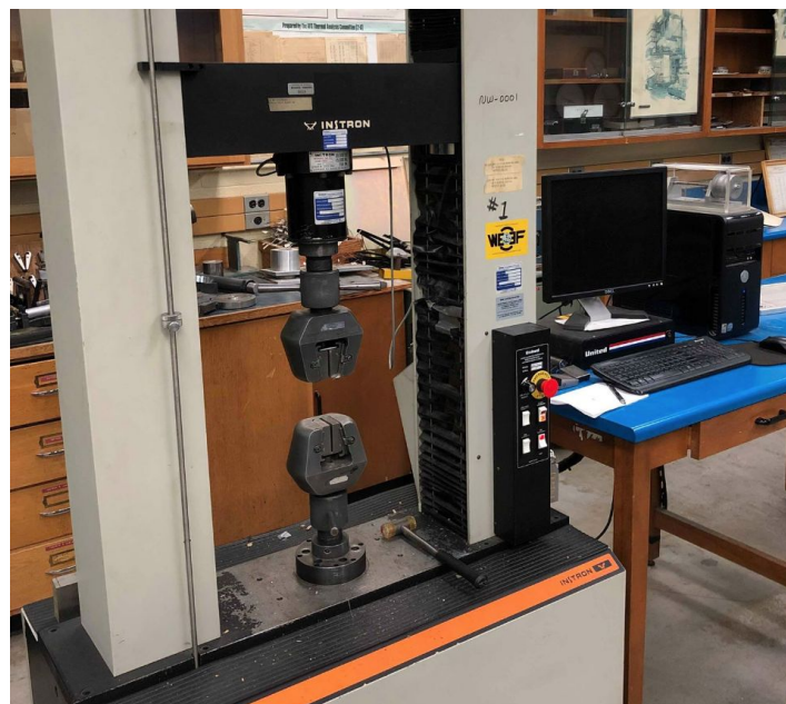
Figure 1: Tensile Test setup on Instron
