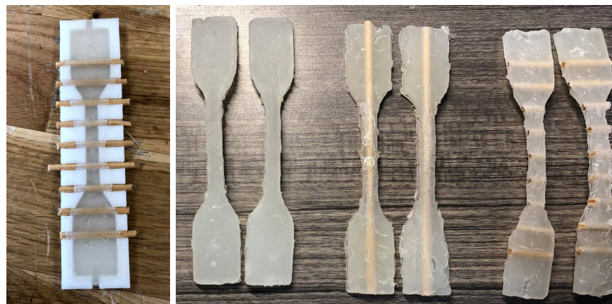
Figure 4: Specimen in mould (left), final specimens for testing (right)
