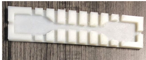
Figure 3: 3D-Printed Composite Mould
