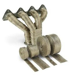
Heating shielding is key in the exhaust systems for a variety of reasons
